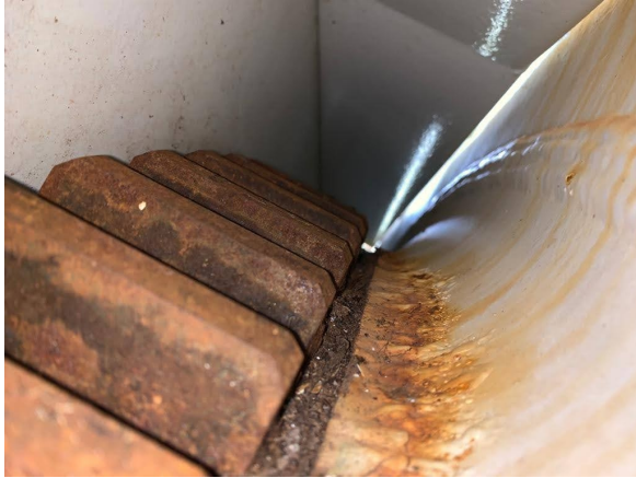
Fig. 4 Rust in RAEGE Santa Maria radiotelescope pinions.
