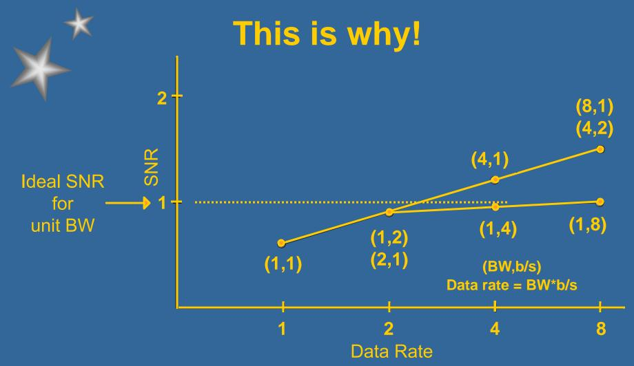
Note that SNR goes up faster by increasing BW than by increasing #bits/sample
