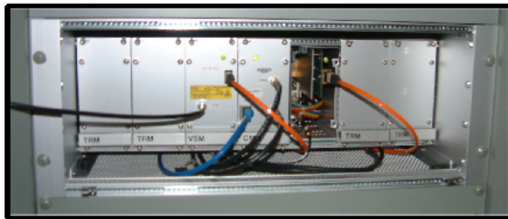
Sampler: 1280 MHz, 8-bit/sample
