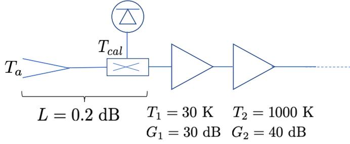
We assume that the physical temperature of lossy components in front of the first amplifier is 20 K. The noise temperatures,  $T_1$  and  $T_2$ , indicated in the figure are referred to the input of the amplifier, and the gains of the amplifiers are denoted  $G_1$  and  $G_2$ . What is the noise temperature of the receiver referred to the antenna input?
