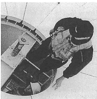
Figure 2. Attaching the antenna mounting device for the GPS-antenna NVTX to the theodolite mount.
