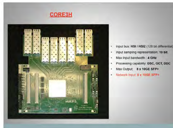
Fig. 3: The FPGA processing board CORE3H can be populated with up to eight optical transceivers. They can work as output (standard DBBC3 VDIF streams for recording) and as input to the FPGA (application for “digital” receivers).
