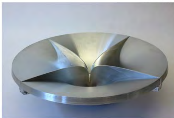
Fig. 5: The manufactured QRFH feed without the dielectric inset. The flatness of the feed is due to the very large opening angle of the Effelsberg telescope of 2 \times 79^\circ .
