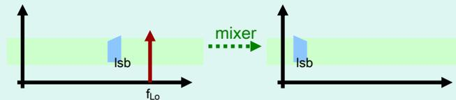
Note that in the lower sideband (lsb) output, the ordering of the frequencies is reversed.
