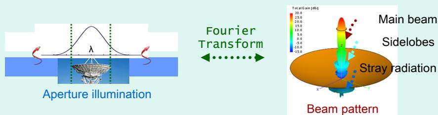
Depending on the details of the aperture illumination, the Half Power Beam Width (HPBW) is approximately
