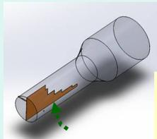
If a septum is inserted in the waveguide both linear polarizations can be combined to get both circular polarizations without the need for external circuitry.
