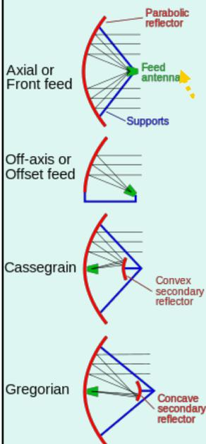
The *purpose of the reflector system* is to concentrate the radiation intercepted by the full aperture (and from the boresite direction) into a single point.
