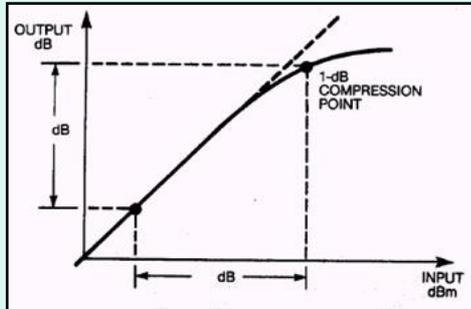
The **1 dB compression point** is an important amplifier specification. It is a measure of how large a signal can be input to an amplifier before significant non-linear behaviour begins. It occurs at the input signal level where output increases 1 dB less than the input. To guarantee linear operation, systems are usually designed to operate at least 10 dB below the 1 dB compression point.
