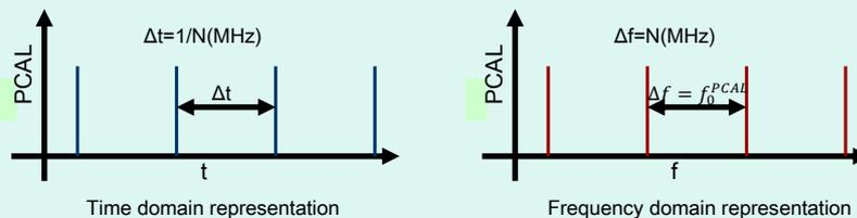
The PCAL signal is detected in the digital output of the receiver (usually at the correlator where it is used). The detection can be either in the time domain or the frequency domain:
