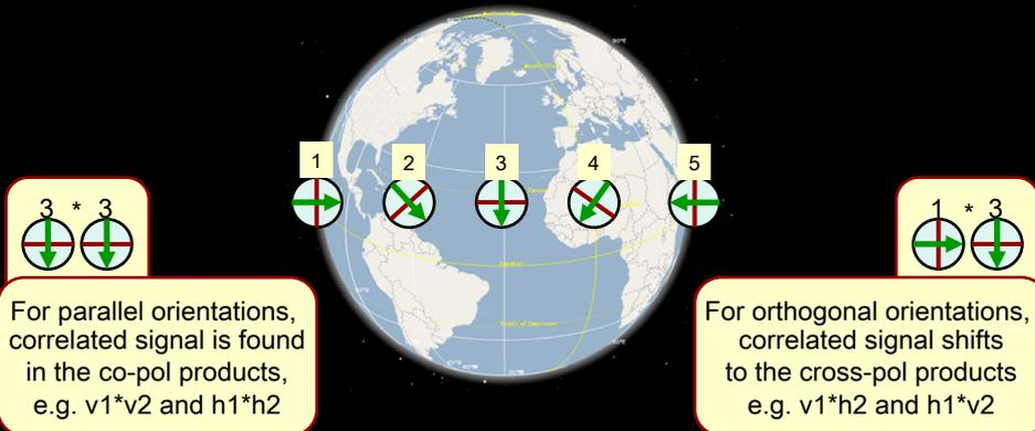
For parallel orientations, correlated signal is found in the co-pol products, e.g.  $v_1 \cdot v_2$  and  $h_1 \cdot h_2$
