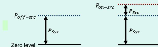
Using  $P_{on-src}$ ,  $P_{off-src}$ , and the flux,  $S_f$ , of the calibration source, SEFD can be determined according to:
