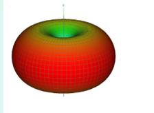
Antenna pattern: Dipole antenna
