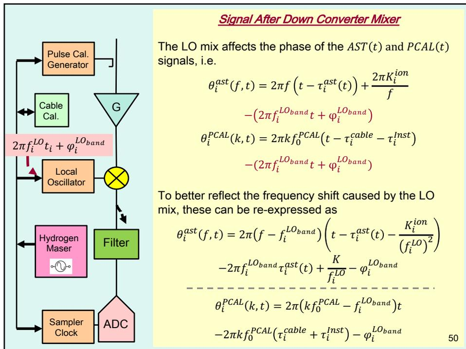
**Signal After Down Converter Filter**
