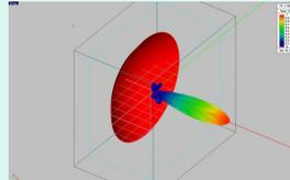
Antenna pattern: Parabolic antenna
