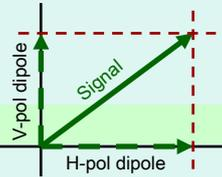
An arbitrary polarization vector decomposed into orthogonal components
