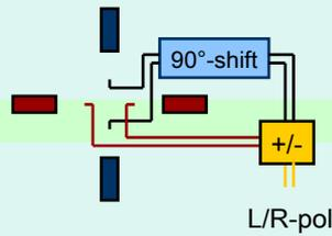
Circular polarization is formed by combining linear signals in quadrature (i.e. by adding and subtracting linear polarizations after one of them has been shifted by 90°). This works easily for narrow band signals – but the existence of broadband 90°-shifters (hybrids) also makes it applicable to broadband signals (like VLBI2010). For this to work well, the electronics must represent the mathematics accurately.
